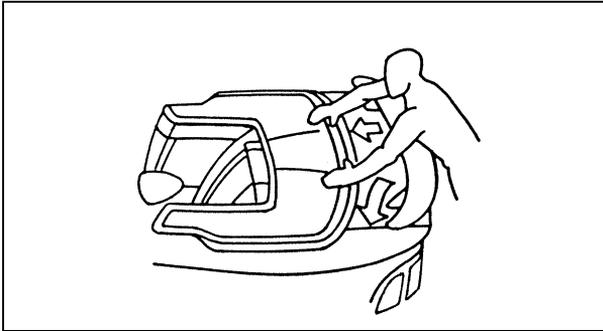
3. Push forward flap of boot until both clips engage under trim panel edge. Repeat on other side of vehicle.
