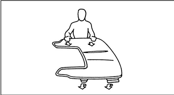
5. Push and pull front of boot to ensure tongue is engaged into groove.
