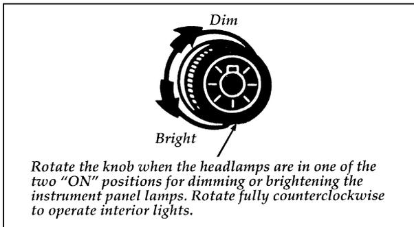
**The knob controls the light on the instrument panel and the interior light**
