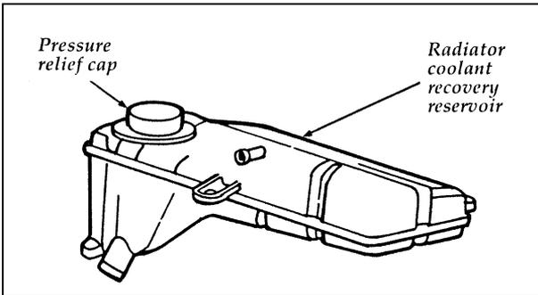
**The engine coolant recovery reservoir — 4.6L engines**
