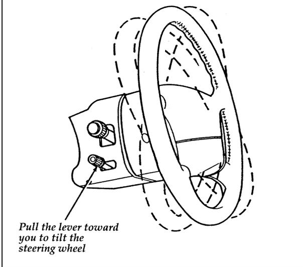
**The lever to tilt the steering wheel**
